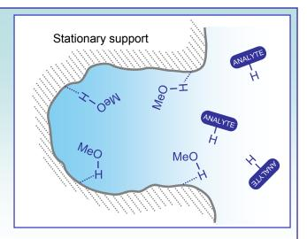
Fig. 1 SHARC surface interacts with hydrogen bonding analytes in acetonitrile (weak solvent) (a); methanol (strong solvent) competes with analytes for stationary phase surface sites (b)
