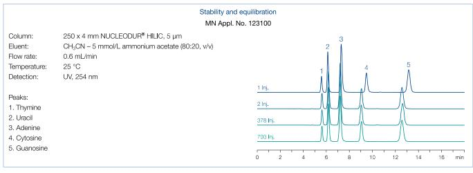
Overall NUCLEODUR® HILIC provides excellent chromatographic features and is hereby the perfect choice for separation of polar or charged compounds which can be shown in application 122920.
