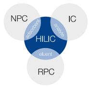
Especially for polar compounds reversed phase HPLC - the most common analytical method - is often limited. Here, hydrophilic stationary phases provide an additional tool for the separation of polar analytes in HPLC.
