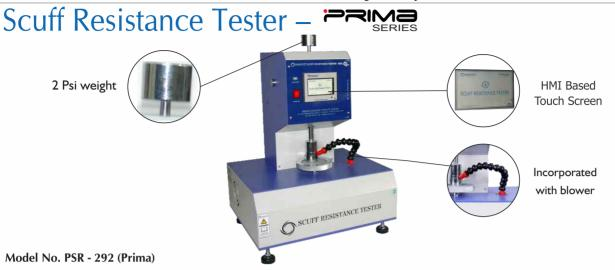
Scuff Resistance Tester Prima Series is a unique test instrument to determine the color transfer from printed or coated material against rubbing. It checks the color transfer when one surface is rubbed against other when subjected to continuous rubbing under specified load. PRESTO Scuff Resistance Tester is designed as per standards ASTM F2497-05, BS 3110:1959. Other model available are Scuff Resistance Tester – Digital Model.
